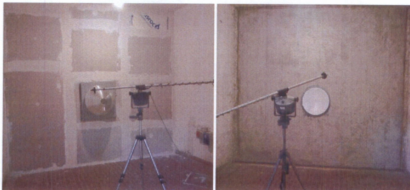
Figure 2 – Specimen under test: source room (left) and receiving room (right).
